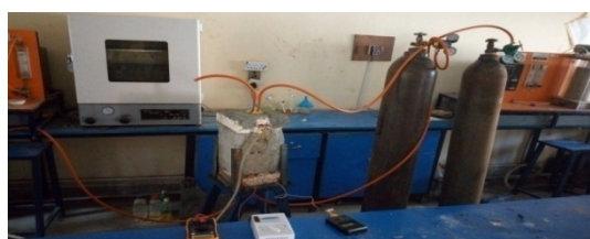
Plate (1): Performance Testing Setup of the DCFC
